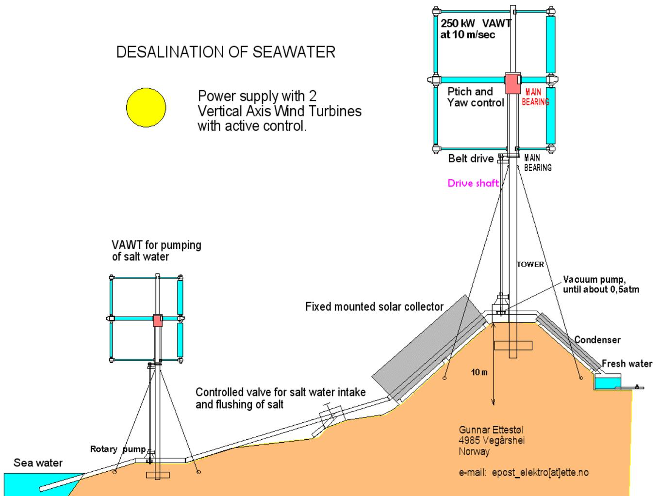
**Wind turbine rotor blades, solar collectors and condensers are made of aluminum and steel and can be easily recycled.**
