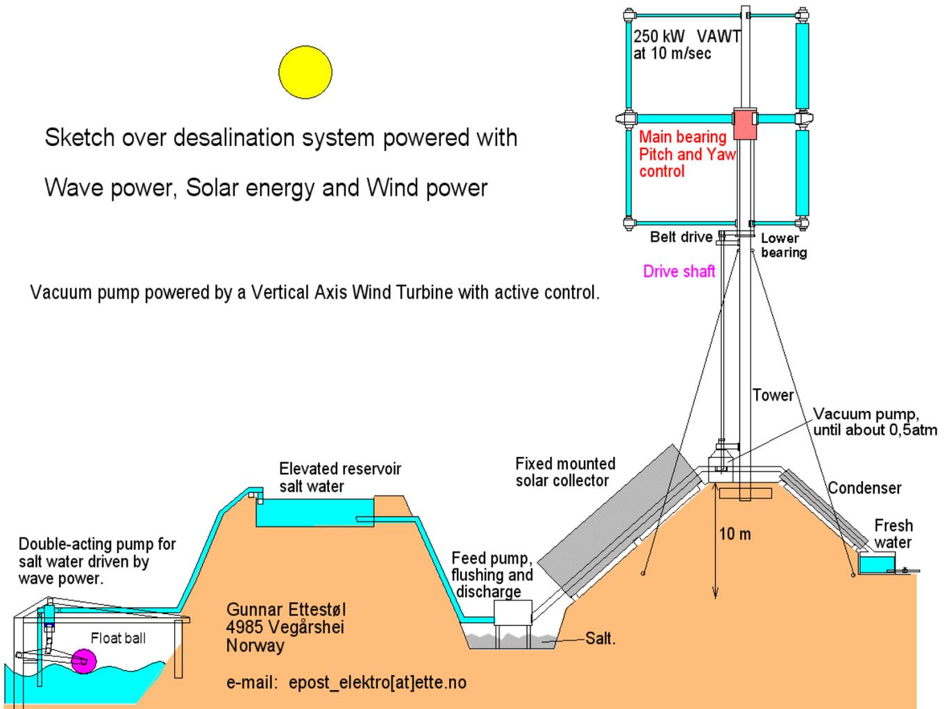
The components in the system above are made from recyclable materials: steel, aluminum and plastic. The rotor blades in the wind turbine are made of aluminum.
