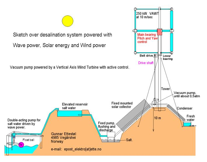
The components in the system above are made from recyclable materials: steel, aluminum and plastic. The rotor blades in the wind turbine are made of aluminum.
